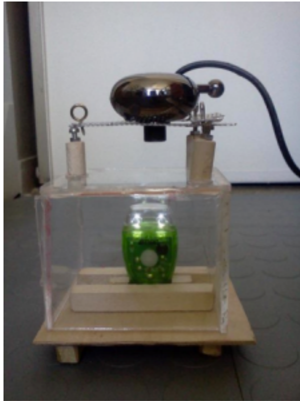
Figure 8: Webcam microscope (with instructions from Hackteria.org)
